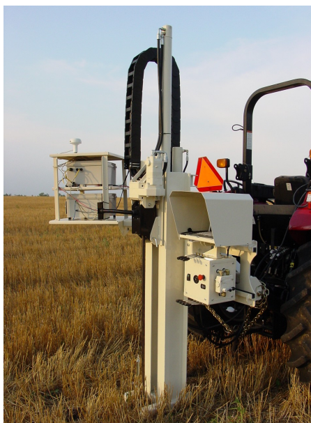
Figure 2. (right) Veris probe-based spectrophotometer for profile measurements.
